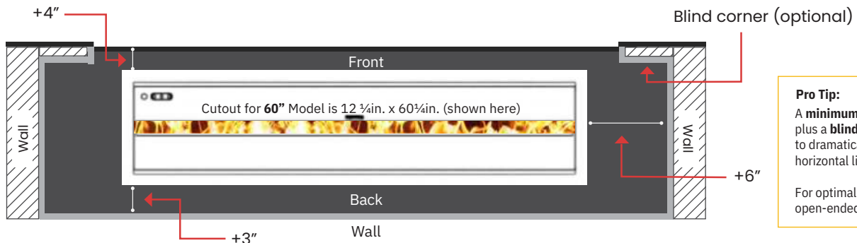
PLAN VIEW SINGLE SIDED & DOUBLE-SIDED HEARTH (walls optional)
